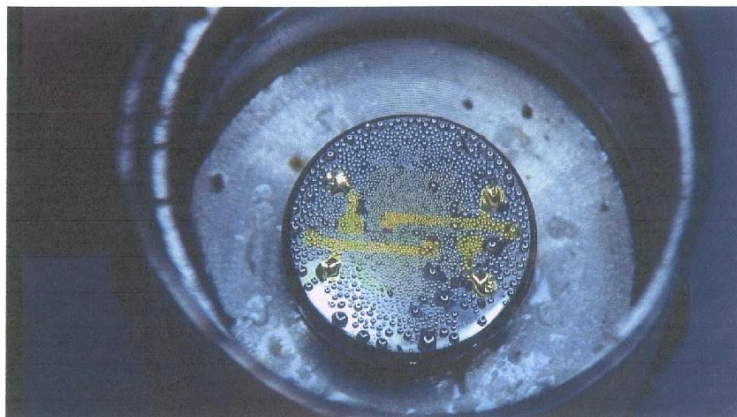
Picture3: moisture on the cell/membrane
